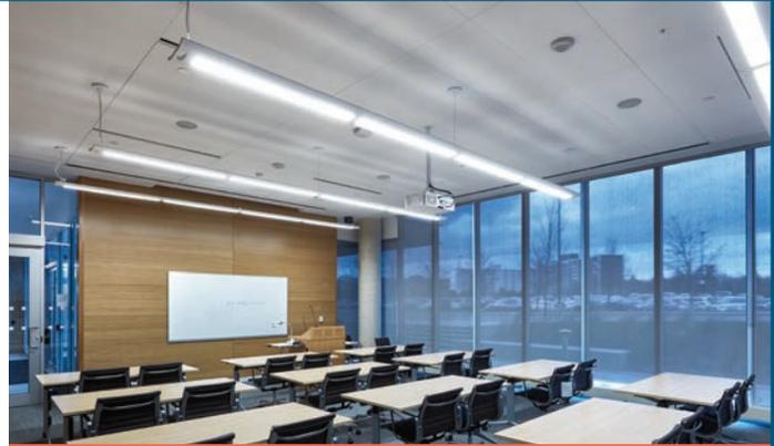
ROCKFON Alaska has an NRC of 0.90 as standard, exceeding performance expectations for ESCB. These stone wool ceiling panels have a high-performing, sound-absorptive material, which can help increase speech intelligibility and improves concentration.
